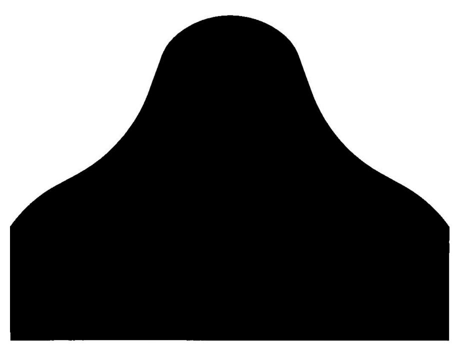
Army F target reduced for 100 yard parctice. Correct dimension for this target is 8.666" wide and 6.333 inches high. Ray-Vin Publishing Co. 2002
