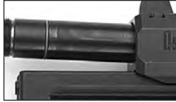
Figure 55 O-ring on barrel
