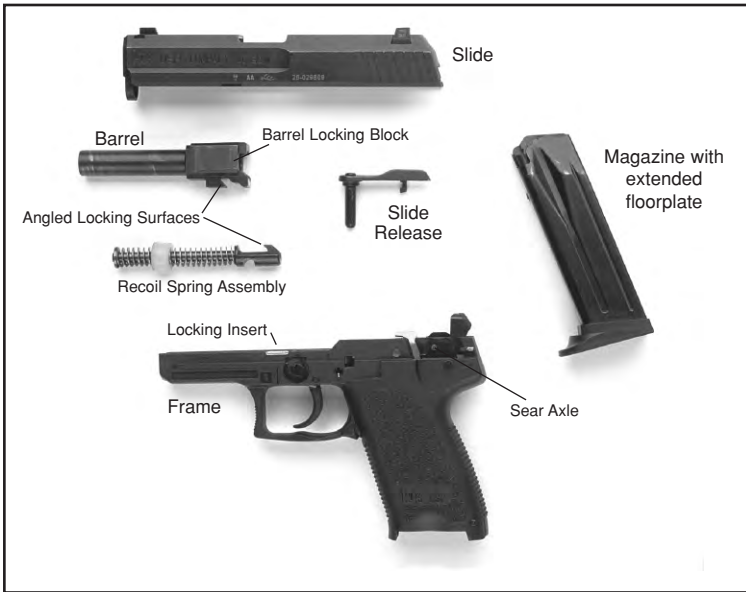
Figure 5 USP Compact-LEM Pistol disassembled (field stripped)
