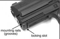
Figure 34 Detail of P2000 mounting rails
