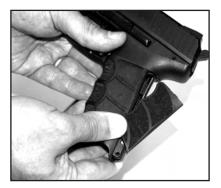
Figure 14 Once the backstrap is removed, simply slide grip panels off the frame.
