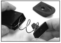
Figure 25 Locking plate and spring
