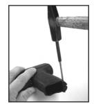
Figure 12 Carefully tap the pin all the way back in.
