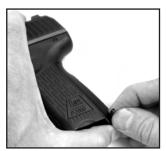
Figure 11 Hold the Grip Panel in place while Inserting the pin.
