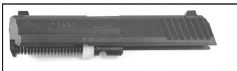
Figure 21 (recoil spring assembly and barrel locking block properly positioned in the slide)
