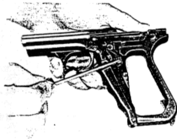
Fig. 17 Engaging rocker spring
