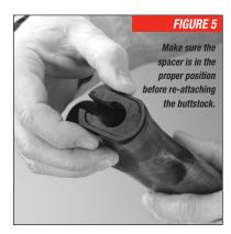
shooters, install this spacer with the R facing out, toward the end of the buttstock, so its thicker side is on the left side of the receiver. This casts the stock slightly to the right, away from the face of a right-handed shooter. Turn the spacer around so the L is facing out and it will cast the stock to the left.
