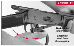
difficult to close the action. Make sure all surfaces are clean if any unusual resistance is felt. However, remember that this is a finely fitted action purposely made with tight fitting tolerances. This assures your gun of good part-to-part fit for many years to come and is the sign of a finely crafted firearm.
