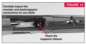
BY LOOKING THROUGH THE TOP OF THE OPEN RECEIVER, THAT THE MAGAZINE FOLLOWER IS SHOWING—AND NOT A SHELL BASE.
