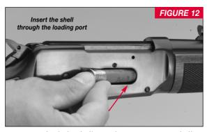
Be sure to check the shell to make sure it is a 24/2" shell and not a 3" shell. If it is a 3" shell do not use it or try to chamber it in your Model 9410. Store it away separately from your gun.
