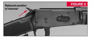
imminent, it is important to lower the hammer immediately to the rebound position from the cocked position. To do this:
