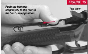
94. It serves to drop an internal hammer block that is positioned between the hammer and receiver. The hammer block prevents the hammer from striking the firing pin until you pull the trigger to fire the rifle.
