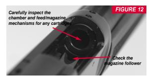
IMPORTANT: ALWAYS VISUALLY NOTE, BY LOOKING THROUGH THE TOP OF THE OPEN RECEIVER, THAT THE MAGAZINE FOLLOWER IS SHOWING — NOT A CARTRIDGE BASE.
