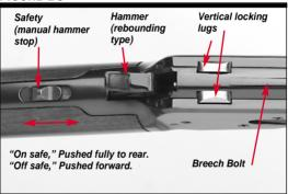
Throughout this manual the "action" refers to the mechanism of this rifle which loads and secures the cartridge in the chamber.
