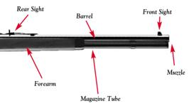
the tubular magazine to the chamber. After firing, working the lever ejects the empty cartridge nearly straight up and slightly to the right, over your head. Returning the lever upward cycles a new cartridge from the magazine into the chamber. The 1892's uncanny, reliable, smooth function made it an instant success in its day. We are sure you will appreciate its incredible design and high level of precision as you become familiar with it by reviewing these instructions.
