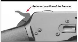
conditions, the hammer is prevented from moving forward and striking the firing pin. The rebound position and the safety (manual hammer stop) are intended to work together to provide protection against unintentional or accidental firing.
