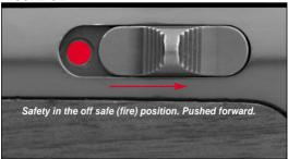
To place the safety (hammer stop) in the "off" position: First, point your rifle in a safe direction, then push the safety fully forward, covering the "S" inscribed on the rifle, and exposing the red warning dot. When the red dot is visible below the safety it is in the "off" position (refer again to Figure 6-B). The safety can be actuated with the hammer in the rebound or cocked position.
