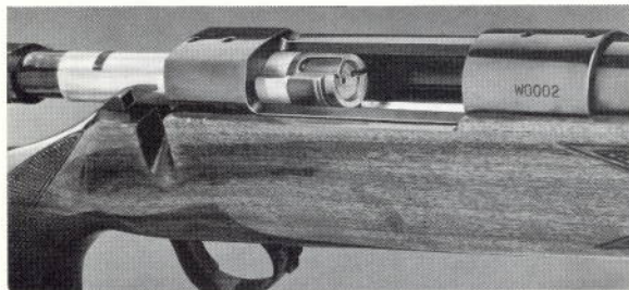
Photo #1: Opened receiver showing recessed bolt face and locking lugs.
