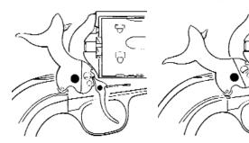
Fig. 3 - 2nd Position Loading Notch
