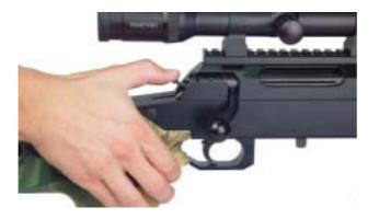
• Press the catch of the bolt and keep it pressed (see picture), at the same time withdraw the bolt towards the rear
