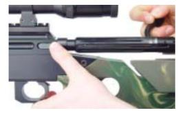
• Release clamp screws of the barrel (SW4) by turning them anticlockwise (see picture).
