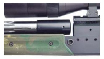
• Open the system with the opposite system screw (SW<sub>3</sub>) by turning it clockwise (see picture).
