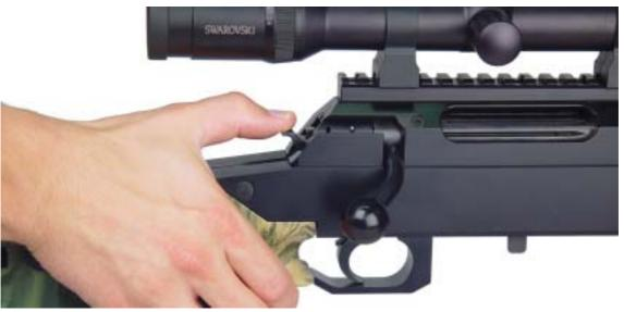
Attention! The rifle safety can be applied cocked and when the bolt is unlocked or withdrawn from the system. The safety cannot be applied with the firing pin forward after a discharged round.
