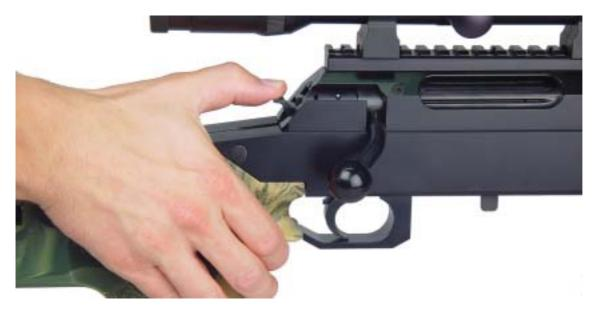
• Remove stock and push bolt catch and keep it down (see picture), at the same time pull the bolt towards the rear.
