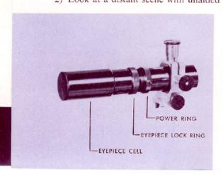
telescope. If properly focused, the crosswires should appear instantly distinct and sharp. If such is not the case, ocular lens requires focusing. It is suggested that the eyepiece cell be unscrewed about ½" from the original position and advanced inward about 2 to 3 turns at a time, until the position is such that the reticule is immediately distinct to the eye.
