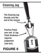
When using the cleaning jag to clean the bore, keep in mind that patch size and thickness are important. Start with a patch that is approximately square (or 2 1/2" round). Position it over the jag as pictured in the illustration and try it in the bore of the firearm (wet patches will enter more easily than dry ones). If it seems to be too tight - don't force it. If your trial patch proves to be too tight, use a smaller size patch and/or thinner material.
