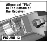
NOTE: Install the breech plug with the "UP" marking on top.
