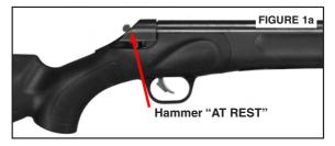
THE HAMMER SHOULD BE IN THE "AT REST" POSITION DURING LOADING AND WHEN CARRYING (Figure 1a).
