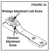
Windage Adjustment Lock Screw (Figure 33). Move the rear sight blade in the direction you want your shots to hit-- (Example; moving the sight blade to the right moves your shots to the right and to the left move the shots to the left).
