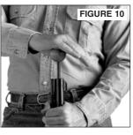
der of the way down the barrel until it contacts the powder charge. The sabot or bullet must be seated firmly against the powder charge. Seat the projectile with the same pressure shot after shot to aid in accuracy.
