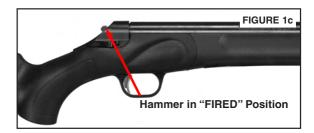
WHEN THE T/C IMPACT IS COCKED AND THE TRIGGER IS PULLED - THE HAMMER CONTACTS THE FIRING PIN (Figure 1c).
