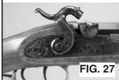
CAP LOCK HAMMER IN “COCKED” POSITION
