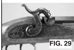
CAP LOCK HAMMER IN “FIRED” POSITION RESTING ON NIPPLE
