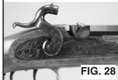
CAP LOCK HAMMER IN “FIRED” POSITION RESTING ON NIPPLE
