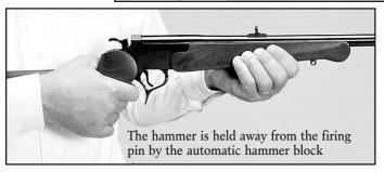
3. Carefully lower the hammer forward, allowing the automatic hammer block to engage in the "at rest" position as shown below.
