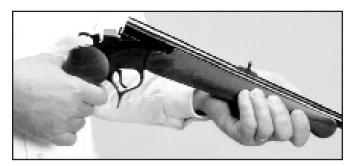
Pulling back on the trigger guard spur will allow the barrel to pivot downward. To close the Encore, pull the barrel upward while securely holding the rifle grip of the Encore stationary with your right hand. Practice opening and closing the Encore before attempting to load and fire this firearm.
