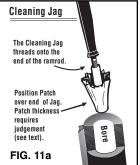
When using the cleaning jag to clean the bore, keep in mind that patch size and thickness are important. Start with a patch that is approximately square (or 2 1/2" round). Position it over the jag as pictured here (Figure 11a) and try it in the bore of the firearm (wet patches will enter more easily than dry ones). If it seems to be too tight - don't force it. If your trial patch proves to be too tight, use a smaller size patch and/or thinner material.
