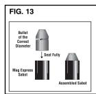
The Assembled Sabot Must Be Seated Firmly On The Powder Charge.
