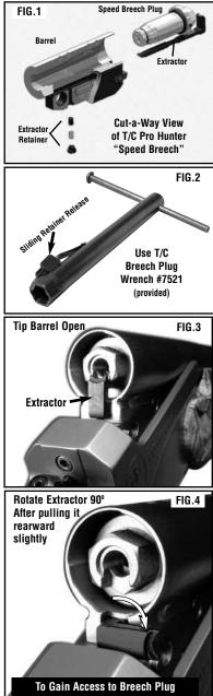
clockwise just 1/4 turn - at which point the extractor is aligned with the extractor slot in the breech plug when the extractor is tipped back into the upright position (see FIG.3).
