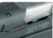
manufactured before July, 2000 do NOT contain a loaded chamber indicator. To determine if chamber is loaded, make sure your finger is not on the trigger or inside the trigger guard and pull slide to rear and visually inspect the chamber. In any case, always inspect the chamber visually by pulling the slide back slowly and looking into the chamber while keeping your finger well clear of the trigger and trigger guard and keeping the muzzle pointed in a safe direction.
