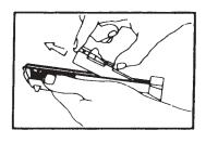
6. Remove the BARREL from the SLIDE.
