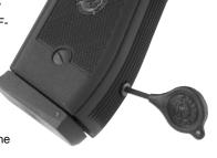
**Engagement (Secure)** PT111, PT111TI, PT132, PT138, PT14O, PT145 & PT145Ti Insert the key into the mechanism and turn clockwise until a click is felt or heard. The mechanism now partially protrudes above the surface of the slide. The action is locked in place and cannot function.
