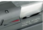
chamber indicator. To determine if chamber is loaded, make sure your finger is not on the trigger or inside the trigger guard and pull slide to rear and visually inspect the chamber. In any case, always inspect the chamber visually by pulling the slide back slowly and looking into the chamber while keeping your finger well clear of the trigger and trigger guard and keeping the muzzle pointed in a safe direction.
