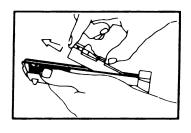
6. Remove the BARREL from the SLIDE.
