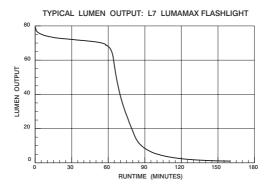
L7 light output if continuously run: 1 hour of tactical-level light, then .5 hour of diminishing moderate light, then 1 hour of minimal light. Total useful light: 2.5+ hours.
