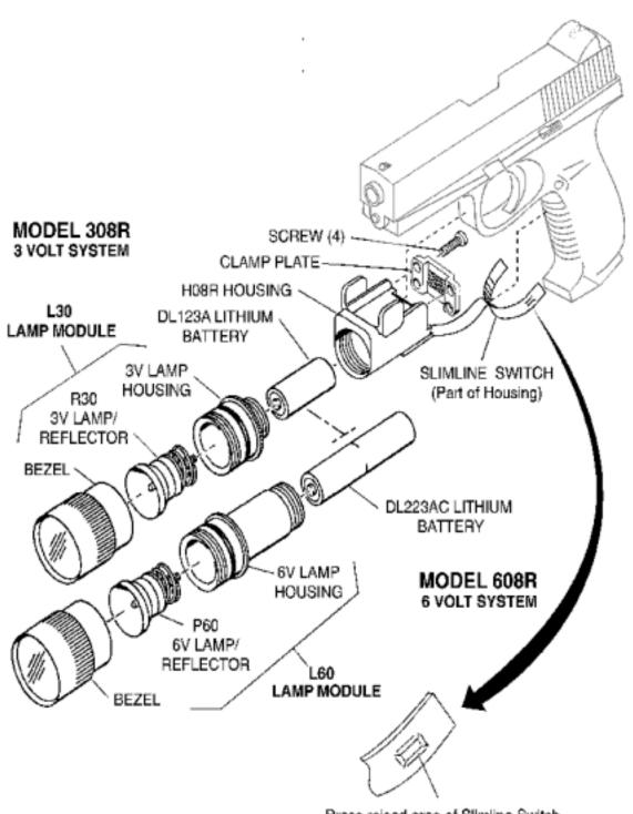
Press raised area of Slimline Switch, LIGHT ON, release LIGHT OFF, Both sides of hand grip.
