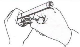
Insert the firing pin, firing pin spring, and locking piece into the bolt head carrier. Depress the locking piece into the carrier, and turn it one quarter turn clockwise.
