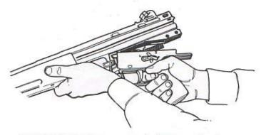
Reinstall the trigger group by first inserting the front of the trigger group, then rolling the rear end with the pistol grip into position.
