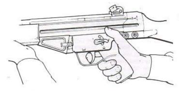
1. Before preparing to use the SAR-3, first make sure the selector lever on the left side of the receiver is in "S" or "Safe" position. While using the SAR-3, the selector lever can be easily manipulated with the thumb of your right hand if you are right-handed or the
