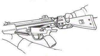
Slide the buttstock back into place over the rear
