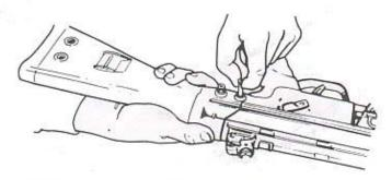
3. Remove the two takedown pins located just forward of the stock. No tools should be required to push the pins through from the right side to the left side of the rifle. When the pins are removed, they should be stored in the small storage holes in the rear of the stock.
