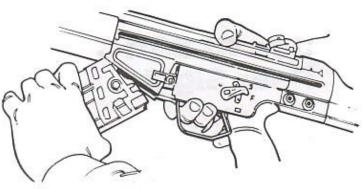
Insert the magazine into the magazine well. The magazine should be inserted, front end first with a slight bottom-forward cant, then rolling the rear of the magazine back into place. When the distinctive "click" of the magazine catch is heard, the magazine is engaged.
