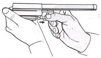
When bolt rollers are depressed bolt assembly should move forward 1/4 "inch.
