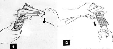
ALWAYS REMOVE THE BARREL RELEASE MECHANISM BEFORE REMOVING THE S.A.S.S.TM SLIDE ASSEMBLY! Serious damage to the S.A.S.S.TM could occur if the release mechanism is not removed before attempting to remove the S.A.S.S.TM slide assembly from the frame.
