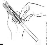
To remove the S.A.S.S.TM barrel, remove the barrel pivot pin from the S.A.S.S.TM slide. The slide stop may be used to help push the pivot pin out.
