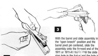
Assemble the S.A.S.S.TM barrel to the S.A.S.S.TM slide by inserting the pivot pin from either side while holding the barrel and slide in proper reference to each other.
