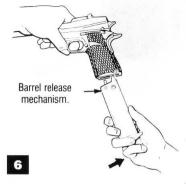
Grasp the barrel release mechanism and pull the barrel release trigger at the bottom half-way back. This will allow the mechanism to slide up into the magazine well without catching or "hanging up." You may also need to press the magazine catch on the frame of the pistol, so the mechanism will
