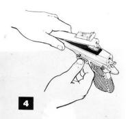
Reinsert the standard slide stop you removed when you disassembled your 1911 or 1911-A1 slide assembly from your frame. If the slide stop cannot be pushed through the aligned holes in the frame and the S.A.S.S.TM slide, you must use a screwdriver to turn the recoil lug adjustment screw. Be sure you use a screwdriver that fits the screw slot properly.
