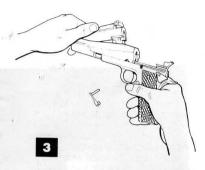
With the action open, remove the slide stop from the frame, then move the S.A.S.S.TM slide assembly forward and off the frame. If the slide does not move forward easily, use extra effort to overcome the tight fitting slide assembly. If necessary, use a rubber mallet to tap on the rer of hte slide assembly, but DO NOT HAMMER ON THE S.A.S.S.TM slide assembly or barrel or the pistol frame and DO NOT PRY WITH ANY TOO!
