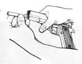
(C) Being careful to prevent the plug from flying out and hitting anyone, gently allow the plug and recoil spring set to move forward. Do not remove set. It will keep the recoil spring guide in place.
