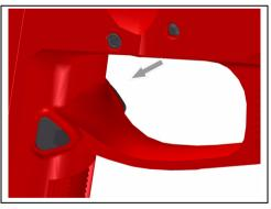
Fig. 5, Pushing in the magazine catch (illustration without trigger)
