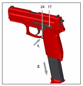
Fig. 3, Removing the magazine
