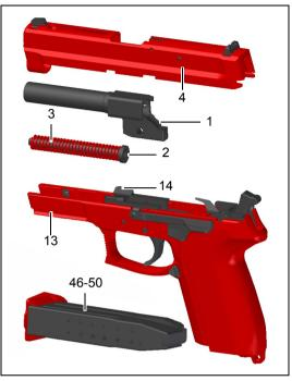
Fig. 17, stripping weapon for cleaning
