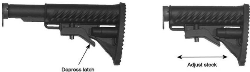
3. To remove the butt stock, pull down on the adjusting latch and remove the stock from the receiver extension.
