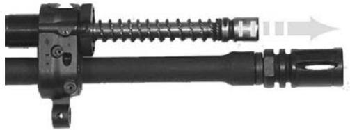
13. Depress the stop pin and rotate the gas tube to the left ninety degrees (90°) until the gas tube notch faces the barrel;
