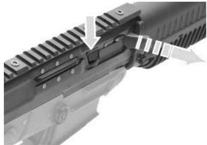
7. Using the charging handle, push the bolt carrier assembly to the rear and remove it from the receiver;
