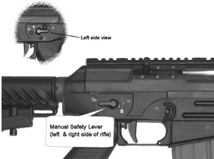
**The safety is “on”** when the safety lever is in the “S” (SAFE) position and the trigger guard is closed. In this position, the rifle cannot be fired with a normal pull of the trigger.
