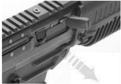
5. Separate the trigger casing from the receiver;
