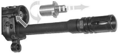
12. Push the operating rod assembly forward and remove from the gas tube;
