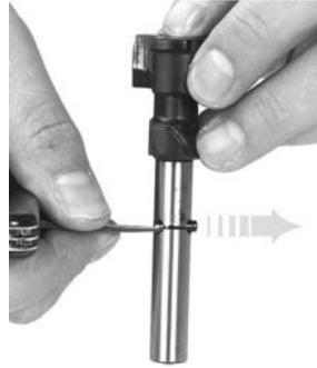
c. Remove firing pin and firing pin spring from the bolt head.
