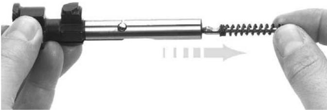
**CAUTION:** The firing pin is under spring tension when installed in the bolt head. Use caution during removal to prevent injury to yourself and others. The use of eye protection is recommended.
