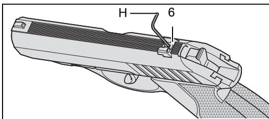
Fig. 4, Slacken and fix the rear sight with Allen key (H)
