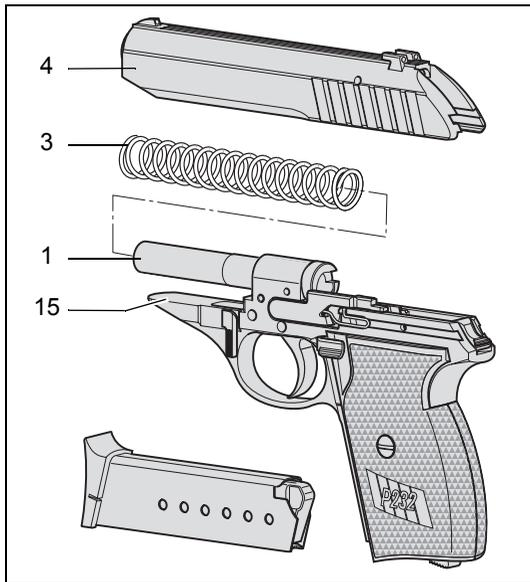
Fig. 12, stripping weapon for cleaning
