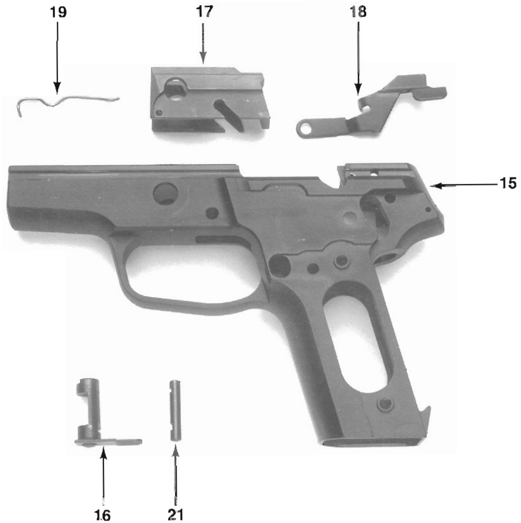
Locking Insert with Slide Catch Lever Spring and Takedown Lever
