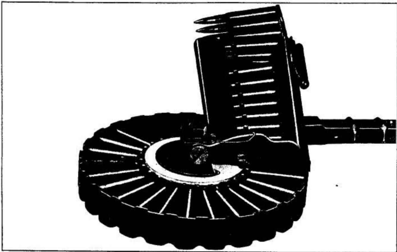
PLATE VIII—LOADING TOOL WITH MAGAZINE IN POSITION
