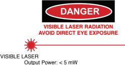
Output Power: < 5 mW Wavelength: 620 - 680nm FDA Class IIIa (IEC Class 3R) Laser Product Complies with 21 CFR 1040.10 and 1040.11 Beam Color: Red
