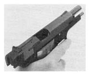
Grasp the slide again and pull it fully to the rear so that the slide stop automatically locks the slide in the open position and remove the magazine. Now you can check the rear of the barrel by viewing it through the opening in the slide to insure that the chamber is empty. If completely empty, your semi-automatic pistol has been rendered clear and safe. You should follow this procedure every time your pistol is handled, inspected, handed to another person or stored.
