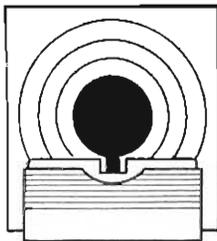
5. LINE the sights carefully, top of front sight even with top of rear notch, and light equal on both sides of front sight (see illustration).
