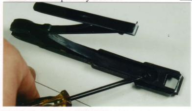
11. After the screw and spring are removed, drift out the cross pin show to remove the arm from the floorplate.
