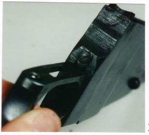
Unscrew the screw and remove the latch down.
