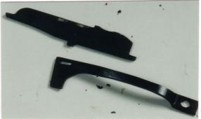
22. The ejector and feed interrupter are on the left side of the barreled assembly. It may be a two-piece or one-piece depending on the model. Unscrew the screw at the rear and drift it forward out of its dovetail. \*Note how the two pieces fit together before disassembly.
