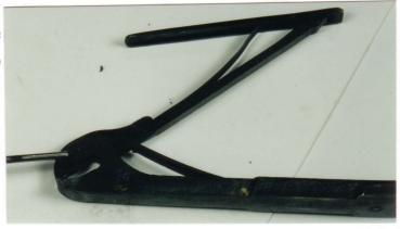
12. Drift this pin out to separate the follower spring and arm.
