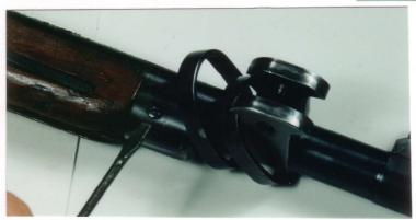
19. The small screw at the front will release the stock cap. This does not need to be removed, unless for repairs.
