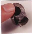
6. The striker is screwed into the cocking knob at the rear of the bolt. Use the forked end
