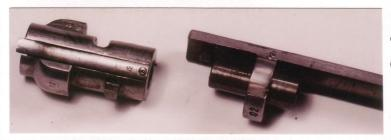
**4.** Turn the bolt head counterclockwise until it stops and remove it.
