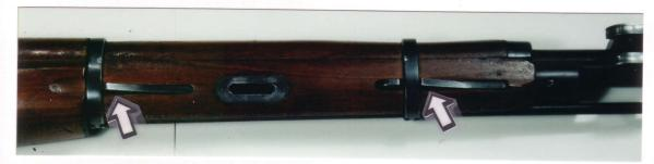
15. If the rifle has a full stock with the upper handguard, push the spring catches and slide the barrel bands forward. The barrel bands will not fit over the bayonet mount. Removal is not recommended(of the sight and bayonet mount). The bands can be stretched slightly. It is recommended that you leave them on, unless for repairs.
