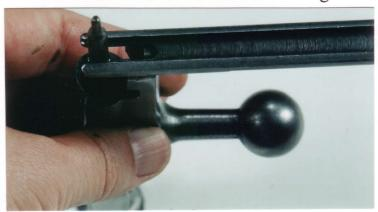
of the bolt connector guide as a wrench to unscrew the striker. It may be tight, do not use force or the bolt connector guide could be broken. It is under tension. As you start to release it keep it under control.
