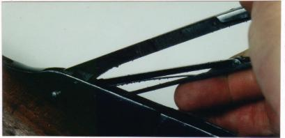
**9.** Squeeze the magazine follower to open the end and remove it back and out.
