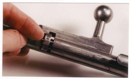
**3.** Slide the bolt connector and bolt head off from the front.
