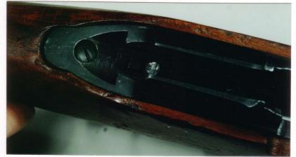
17. To remove the stock, unscrew the large at the top rear of the gun.
