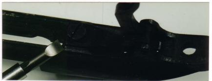
23. Unscrew the large screw underneath the barreled assembly. The trigger spring/bolt stop will not be removed at this time.
