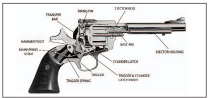
Mechanism shown with trigger pulled and hammer beginning to fall. Transfer bar is in firing position, between hammer and firing pin.
