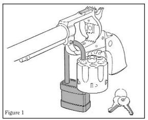
Correct Installation of Lock For Ruger<sup>®</sup> New Vaquero Revolvers (New Model Blackhawk Shown)
