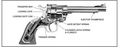
Mechanism shown at rest. Transfer bar is not in line between hammer and firing pin. This is the carrying position.
