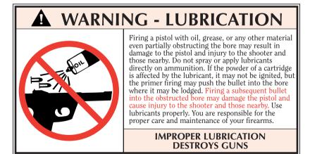
5. Before firing, remove all oil and grease from the bore. Do not keep the pistol stored in a leather holster or case. Leather attracts moisture, even though the holster or case may appear to be perfectly dry.
