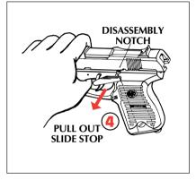
**FIGURE 3** Slide stop in disassembly position.
