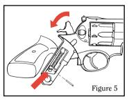
2. Using a properly fitting screwdriver, remove grip screw. Remove pistol grip inserts from grips. Grip panel locator may then be removed. Pull grip downward off frame. Take care not to lose the disassembly pin, which may fall free when the grip is removed.
