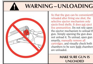
So that the gun can be conveniently reloaded after firing one shot, the selective ejector mechanism only ejects fired shells. It does not eject live ammunition. Do not rely upon the ejector mechanism to unload the gun. Simply opening the gun does not unload it. To unload, open gun smartly, manually remove all cartridges, and visually check both chambers to be sure both chambers are unloaded.
