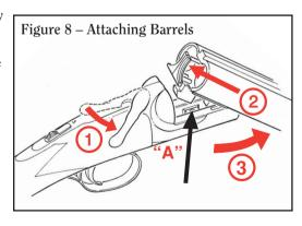
recesses at the front end of the monobloc. Be sure the small lug (indicated by the arrow in "A" in Figure 8.) on the outer surfaces of the ejectors engage the corresponding slot inside the front end of the receiver *BEFORE CLOSING* THE GUN! The foregoing caution must be followed otherwise the receiver will be damaged by the ejectors as the gun is closed.
