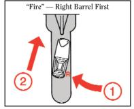
Figure 6. Safety selector in forward "Fire Right Barrel (R) First" position. Pulling the trigger will fire the right barrel – a second pull will then fire the left barrel. It is not necessary to select between shots. The safety selector should be in this position only when the gun user is actually firing.
