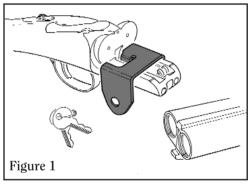
Correct Installation of Clamp
