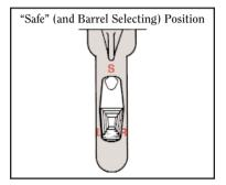
Figure 4. Safety selector in "Safe" (S) full rearward position. The safety selector must be in this position to select position 'L' or 'R' described below. In this position, the trigger cannot be pulled to fire the gun. Either 'L' or 'R' may be partially visible, but the shotgun is only on "Safe" when the 'S' is fully exposed. If the 'S' is not visible, the shotgun is ready to fire!
