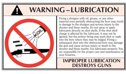
PERIODIC MAINTENANCE – At regular intervals, or whenever the gun has been exposed to sand, dust, extreme humidity, condensation, immersion in water, or other adverse conditions, take down and clean and oil as outlined above. Lubricate contact area of forend iron and receiver with Stainless steel lubricant. Proper periodic maintenance is essential to the reliable functioning of any firearm.
