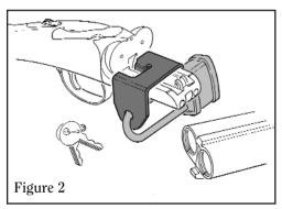
Correct Installation of Lock through Clamp For Ruger Side By Side Shotgun <u>Only</u>
