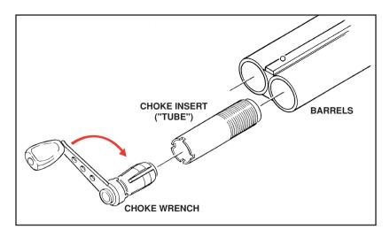
NOTE: *Stainless Steel* choke inserts may protrude slightly from muzzle when fully seated. This is normal and helps protect the muzzle of the barrel from damage.
