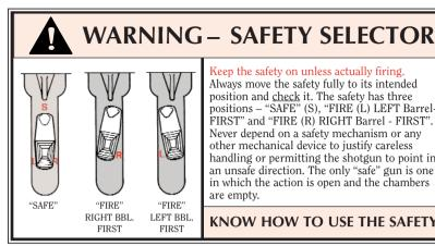
Keep the safety on unless actually firing. Always move the safety fully to its intended position and check it. The safety has three positions - "SAFE" (S), "FIRE (L) LEFT Barrel-FIRST" and "FIRE (R) RIGHT Barrel - FIRST". Never depend on a safety mechanism or any other mechanical device to justify careless handling or permitting the shotgun to point in an unsafe direction. The only "safe" gun is one in which the action is open and the chambers are empty.
