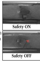
to the right and is perpendicular to the barrel and the green "S" is exposed, the rifle will not fire when the trigger is pulled.
