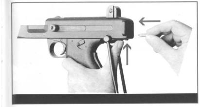
Detachment of the lower sub-assembly: safety latch is pushed upwards then using a pointing object, the latch is pushed inwards and the same time the rear end of the sub-assembly is pulled away from the receiver.
