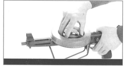
Cocking the drum driving spring: the spring mechanism is turned in clockwise direction.
