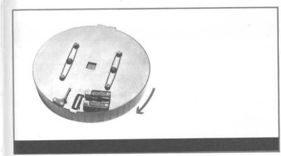
Inserting the cartridges into the drum.
