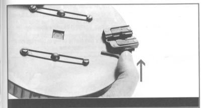
Removing the cartridge guide fixed to the drum plate.
