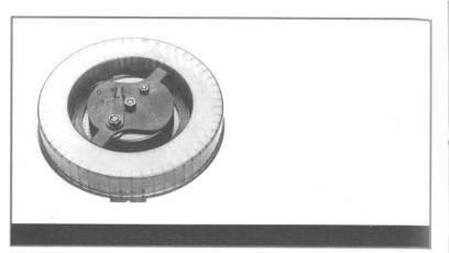
Spring mechanism safety. Hand in position  $\infty$  — driving spring released. Hand in position 0 — driving spring blocked.
