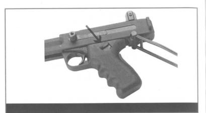
Manual safety: when pointing to the rear, the weapon is on "safe", but when the lever points towards the trigger, firing is possible.
