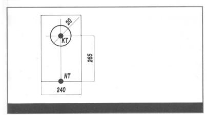
NT-the aiming point, KT- the control point
