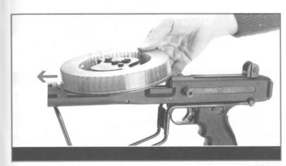
Drum placement: wide protrusion of the drum plate forward end is pushed into the notch in the drum bed forward end.
