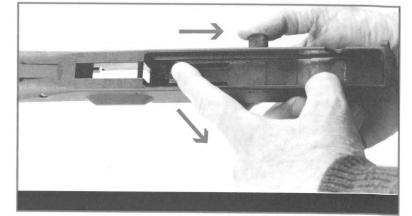
Pulling the bolt out of the receiver. The arrows indicate the direction of the movements.
