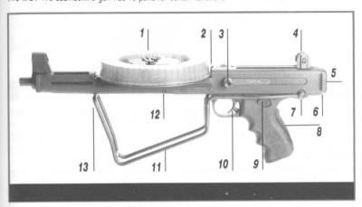
1 - drum spring mechanism, 2 - drum latch, 3 - cocking handle, 4 -adjustable rear sight, 5 - lower sub-assembly latch, 6 - safety button for lover sub-assembly latch, 7 - stock latch, 8 - automatic safety, 9 - manual safety, 10 - trigger, 11 - folding stock, 12 - barrel holder, 13 - folded stock latch. Manipulation with individual operating parts is specified in the next chapter.
