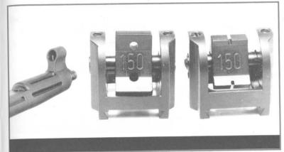
The MGV 176 has a fixed front sight with protective tunnel and the adjustable rear sight in two versions. The rear sight basic configuration has three folding leaves with notches for firing at a distance of 100, 150 and 200 m. These numbers are marked on corresponding leaves. A spring-loaded latch holds the three-leave folding piece in set position.
