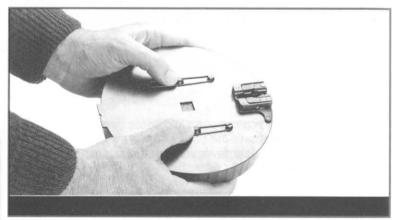
Detaching the spring mechanism from the drum plate.
