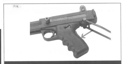
Automatic safety is formed as a squeeze-lever on the back of the grip. The shooter disengages it automatically when correctly holding the gun grip; when he abates the grip, the safety automatically puts the mechanism on "safe". This way the automatic safety prevents activating the gun when it falls down accidentally and in similar situations.
