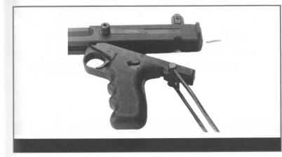
Lower sub-assembly separated from the receiver
