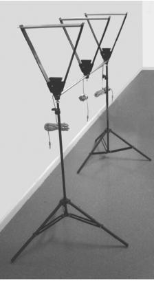
Use the 4' rail with a light stand under each end. Mount start and stop skyscreens using a 3" threaded stud with attached wingnut as the mounting screw. The long tail of each stud slips into the hollow center post of a stand. Make sure that the screws fit into the dimples of the rail. Tighten each thumbscrew and stud firmly by hand.
