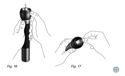
**3.** Grasp the lamp firmly (Fig. 17) with thumb and forefinger. Pull straight up until lamp's pins are clear of receptacle. Do not dispose of old lamp in fire or trash compactor.
