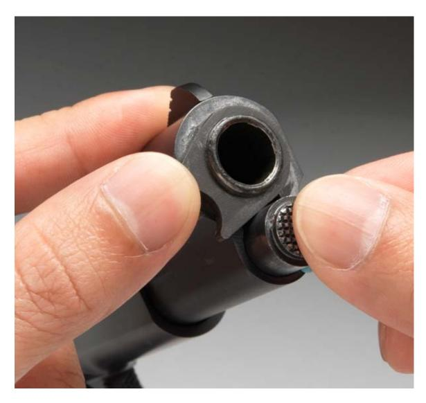
Figure 5. Remove the Recoil Spring Plug
