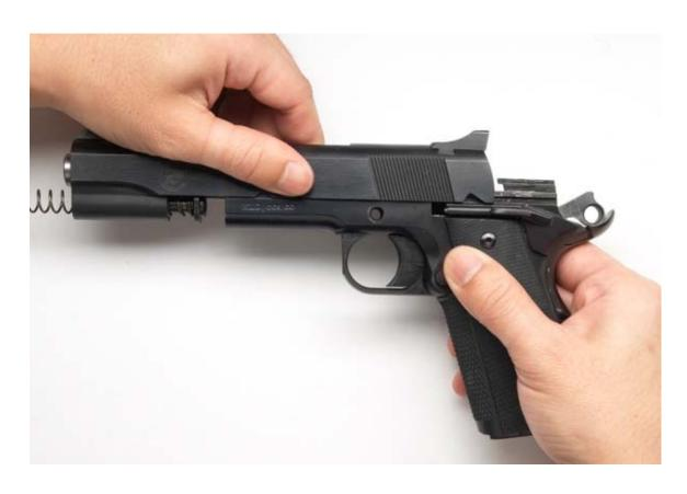
Fig. 7 Remove the Slide
