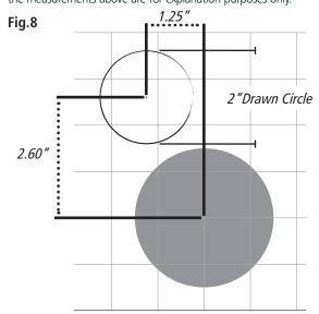
Note: When recreating your total offset on the alignment aid, remember that the horizontal distance should be marked as though you were behind the bow/sight. Using the example above, the Vendetta would be to the left of the top pin when viewed from behind in a firing position.
