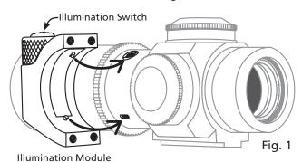
4. Align the other half of the module with the 4 screw holes
