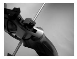
Adjusting the Single-Action trigger weight Simultaneously Left side - hold the trigger spring stud screw Right side - loosen the secondary side screw, then adjust the trigger spring stud screw slightly and retighten the right side clamp screw.
