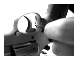
Adjusting the trigger stop screw
