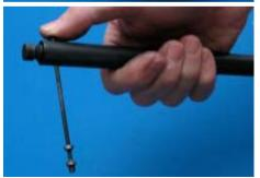
now free to be taken off. Slide the recoil spring tube off the piston rod and remove the recoil spring from the recoil spring tube.
