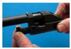
spring tube so that the locking tab points towards the top of the bolt carrier. Check the operation of the recoil spring by lightly pulling on the recoil spring tube to compress the spring.
