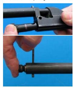
now be able to be pulled straight out of the bolt carrier. After the operating handle is removed the bolt carrier assembly can now be guided out of the bottom of the receiver by holding onto the recoil spring tube.
