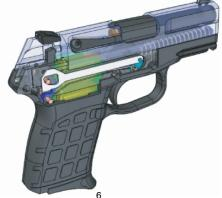
Close to the rear position, the empty case hits the ejector, and is thrown out of the gun. The recoil springs drive the slide forward again. The top cartridge in the magazine is picked up by the breech face and pushed into the barrel. Close to battery, the barrel is cammed up, positively locking into the slide.
