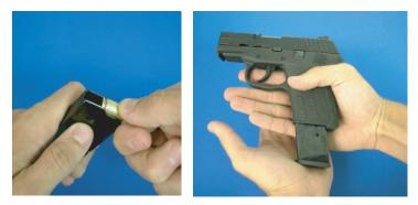
Hold the pistol in one hand with the muzzle pointing in a safe direction and with your finger off the trigger and outside the trigger guard. Insert the loaded magazine into the grip until it is locked in place. Check to assure magazine is secure. Pull the slide back and release. This strips a round from the magazine and seats it in the barrel chamber. At all times keep your hands away from the muzzle.
