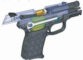
During the rear recoil motion, the hammer is disengaged and follows the slide, acting like an extra recoil spring. As the slide moves forward, the hammer rotates with it until the hammer block reengages the hammer, holding it away from the firing pin. When the trigger is released the trigger bar moves backwards and behind the hammer catch. The pistol is then ready for the next shot.
