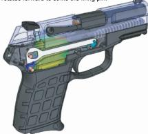
The ignited powder gas drives the bullet forward through the barrel and simultaneously drives the slide and barrel backwards. After about 1/4" (6 mm), the barrel is unlocked by the assembly pin and releases the slide to travel back, extracting the case. On it's way back, the slide is gradually slowed down by the recoil springs.
