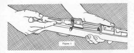
TO OPERATE: When gun is fired raise the bolt handle and pull back sharply to the rear as far as it will go. Push the bolt forward and the bolt handle down to load the gun. Always push safety on safe to prevent accidental firing.
