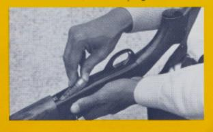
To unload magazine, depress carrier latch button and push carrier plate down. Holding shell stop with thumb, remove shells from magazine. To unload chamber, pull back charging handle. Note: All shells may be removed by pulling back charging handle and cycling shells from magazine to chamber.
