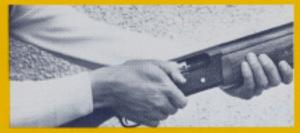
15. To load chamber, pull back charging handle until action remains open. Insert shell into loading port of receiver and slowly close action. Note: A round will feed from magazine to chamber when charging handle is pulled back by hand.
