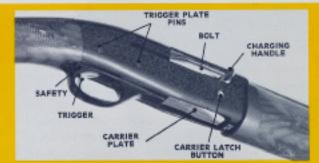
Put the safety in the "ON" position (Red Band Hidden). Check chamber and magazine for
