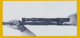
With the bolt still in the open position slide the barrel ring over the magazine tube and barrel into the receiver. Be sure the barrel is fully seated in the receiver.
