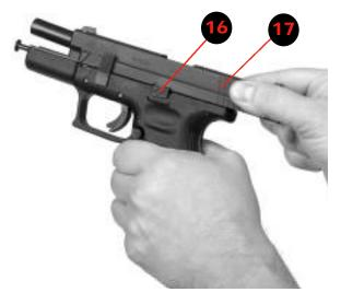
Now slip the complete assembly {slide (17), barrel (18) and dual tension recoil spring (19)} forward and off the frame (20).
